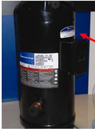
Figure 14: Advanced Scroll Temperature Protection (ASTP)
